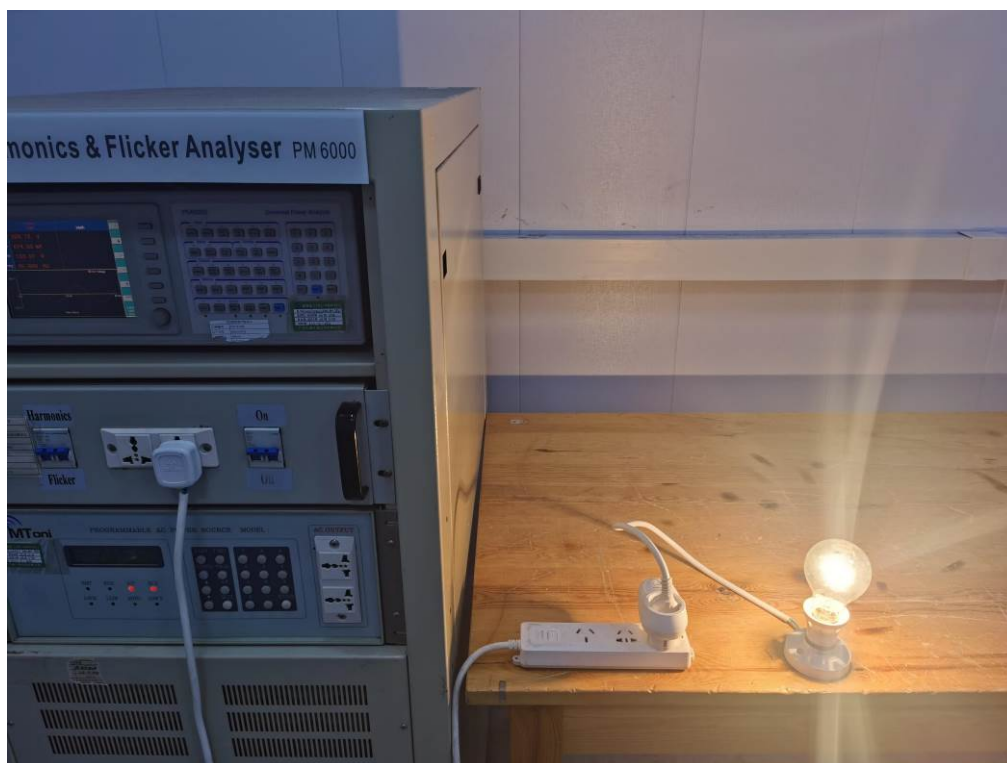
Voltage Fluctuations and Flicker
