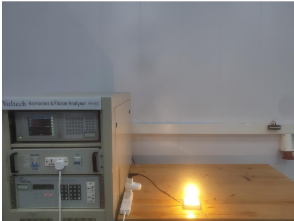
Voltage Fluctuations and Flicker
