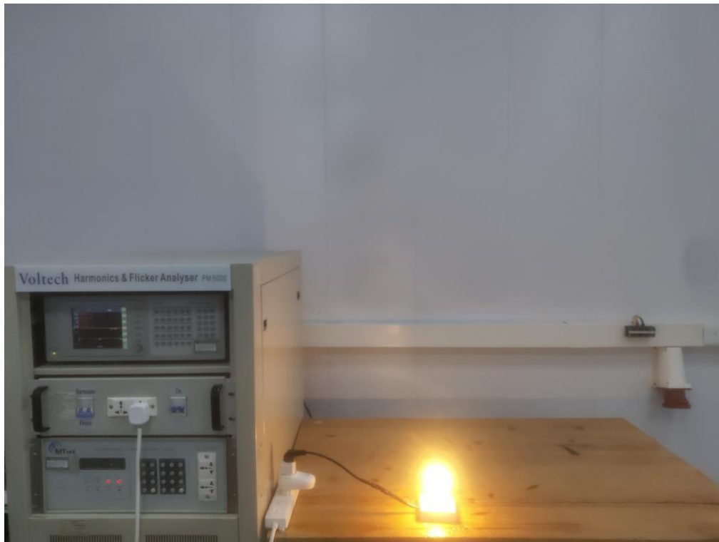
Voltage Fluctuations and Flicker
